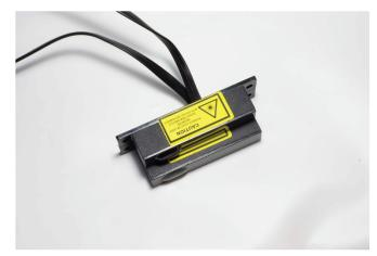
Outer sensors (see picture above) can be mounted in horizontal or vertical position, important is that sensors have a unobstructed "view" of road front and back (mounting behind plastic, metal, or glass objects including grills is NOT a option).
